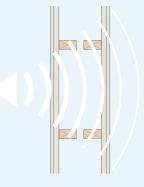
In an unfilled cavity, the plasterboard linings and cavity alone provide the sound insulation which can result in poo performance and a hollow sounding construction.
